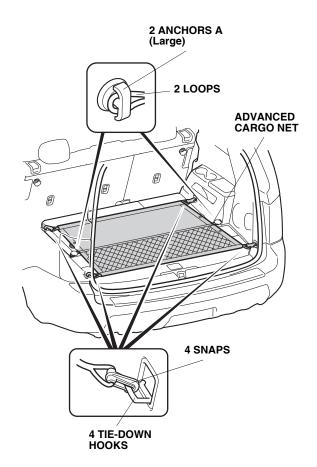
26. Attach the four snaps on the advanced cargo net to four tie-down hooks. Hook two loops on the advanced cargo net to the two anchors A (Large) on the third row seat back board.
