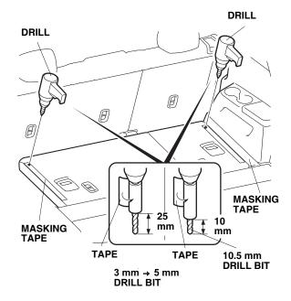
7. Enlarge the holes with a 10.5 mm drill bit. To drill through the hard board only, wrap tape around the drill bit 10 mm from the tip as shown.
