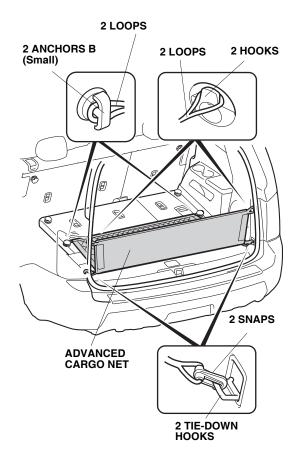
29. Attach the two snaps on the advanced cargo net to two tie-down hooks.
