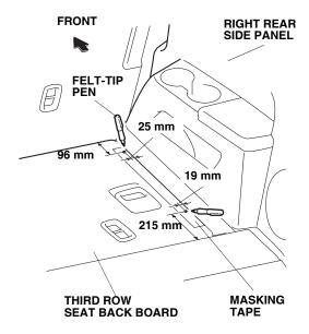
5. Using a felt-tip pen, measure and mark two locations on the masking tape.
